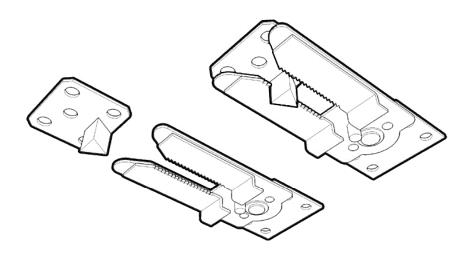
To release, lift the unit with clip A attached up and away from the adjoining unit.
